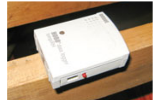
Figure 5. Readouts from Hobo data loggers placed in the building (photo, right) indicated high humidity in the crawspace (above left), with air temperatures only slightly higher than dewpoint temperatures, creating a risk of condensation. Upstairs humidity was also high — typical for an unconditioned building in the summertime — but the average temperature stayed well above dewpoint (above right).
